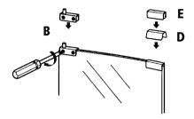
Push the top glass door hinge into the top right bushing and gently slide the glass door into the bottom hinge. Adjust the glass door until level, and tighten the hinge screws.
